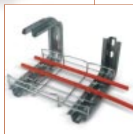
pyrosys® Cable trays and cable ladders E30/E90 Spacing ≤ 1500mm
