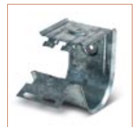
pyrosys® Multi cable support "Hermanschelle" E30/E90 Spacing ≤ 600/800mm
